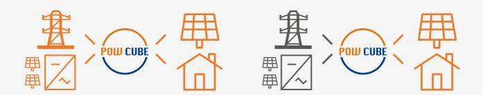
With the Sungrow meter installed, the system could be configured to a zero-export or partial-export system to meet the utility grid restriction. In this case, the inverter output will adjust to match the load consumption power continuously to restrict the export power.
